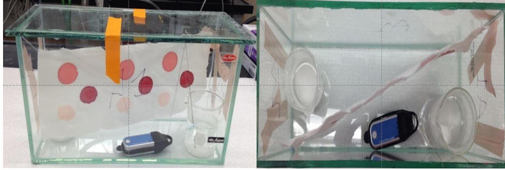
Figure 1.5. Artificial aging environment created with glass tanks (side and top views).
